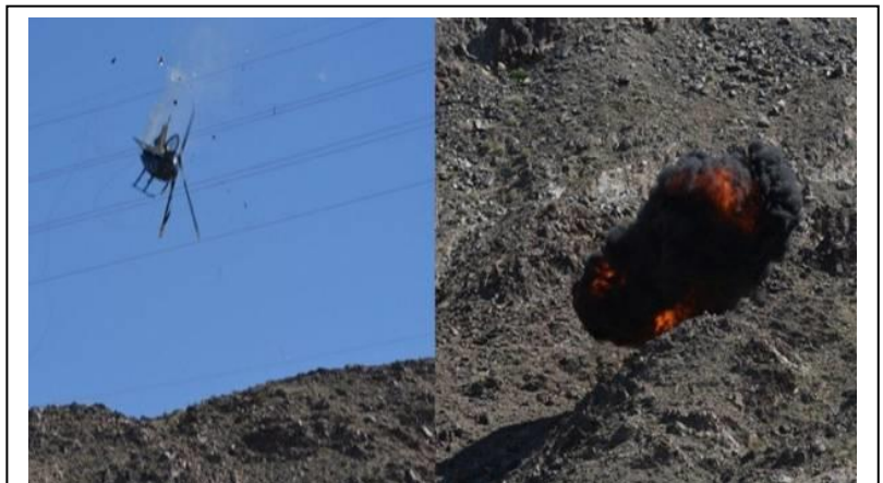
Four rescuers were killed in the crash of this helicopter when it encountered power lines during a body recovery of a deceased hiker.
